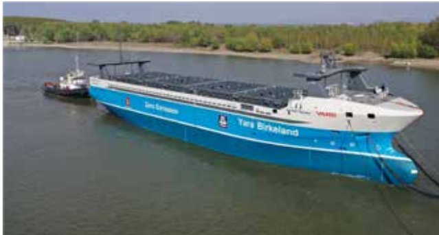
Yara Birkeland the world's first autonomous and zero-emission container vessel. Photo: Kongsberggruppen, Yara
